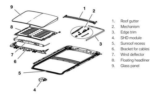
The cables of the sunroof cassette cannot be serviced individually, if they are defective, the entire cassette must be replaced. If the sliding/tilt lever is damaged the cassette must also be replaced.
